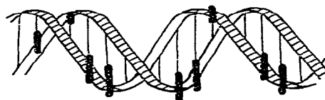
Fig. 3. Schematic drawing of the suggested model of the DNA-caffeine complex: external binding of stacked caffeine molecules in one of the grooves of DNA.
